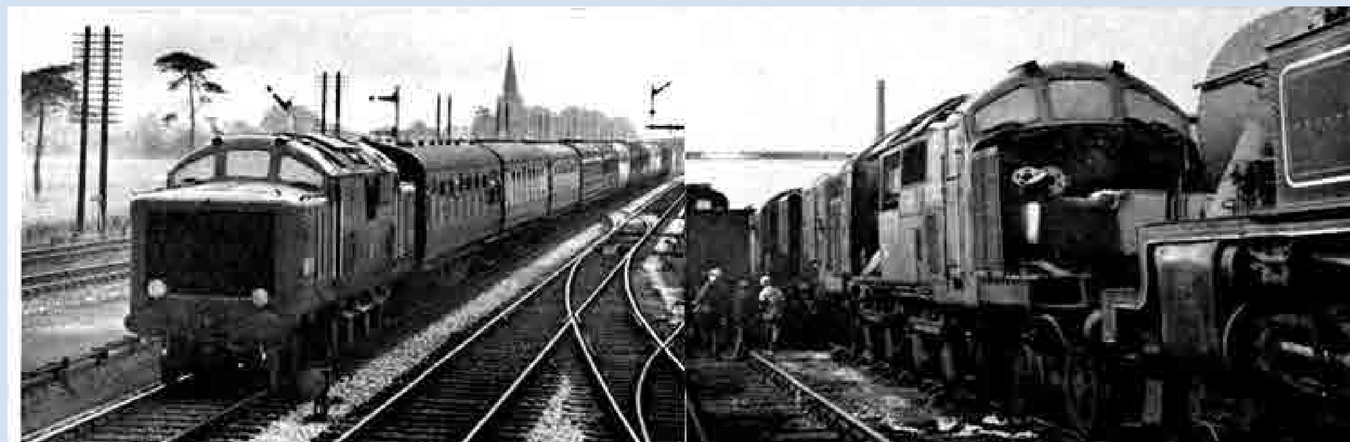
LEFT 10100. The 'FELL' 2,000 h.p. experimental diesel-mechanical locomotive hauling a 12-coach train past Duffield between Derby and Manchester while undergoing trials in 1955 RIGHT April 21st 1960 saw it in the scrap yards at Derby, its power equipment has been removed whilst behind it is 10800 an 827 h.p. diesel-electric built in 1950 by contractors.
