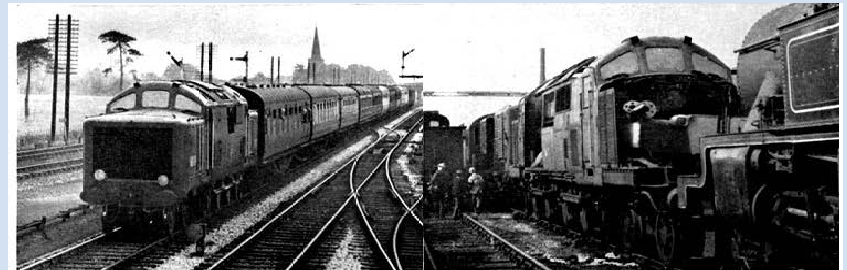
LEFT 10100. The 'FELL' 2,000 h.p. experimental diesel-mechanical locomotive hauling a 12-coach train past Duffield between Derby and Manchester while undergoing trials in 1955 RIGHT April 21st 1960 saw it in the scrap yards at Derby, its power equipment has been removed whilst behind it is 10800 an 827 h.p. diesel-electric built in 1950 by contractors.
