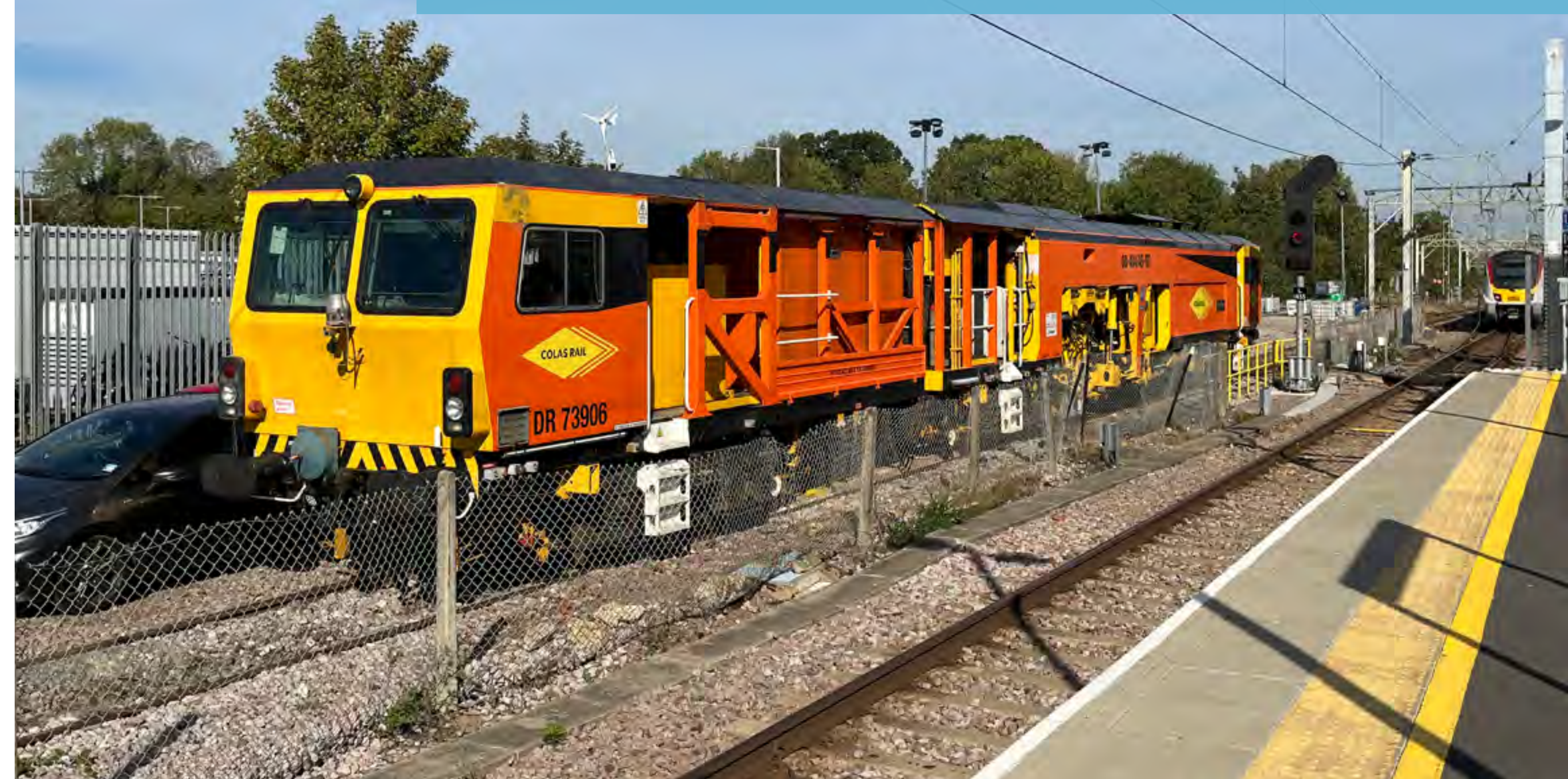
Colas Rail tamper No. DR73906 is seen stabled in Broxbourne Tamper Sidings on October 10th. Derek Elston
