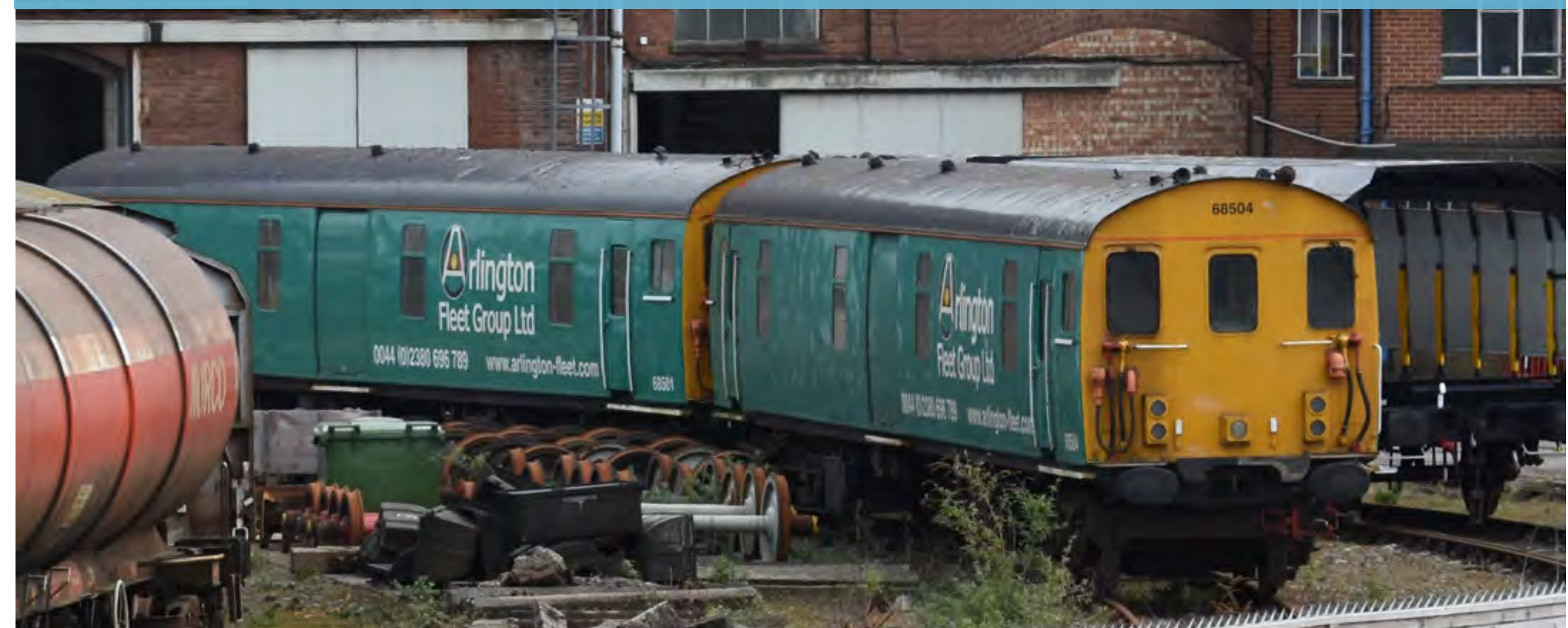
Nos. 68501 and 68504 are former Class 489 Gatwick Express motor luggage vans and subsequently de-icing units which are now converted to Arlington Fleet Services EMU translator vans and are seen outside Eastleigh Works on April 26th. John Sloane
