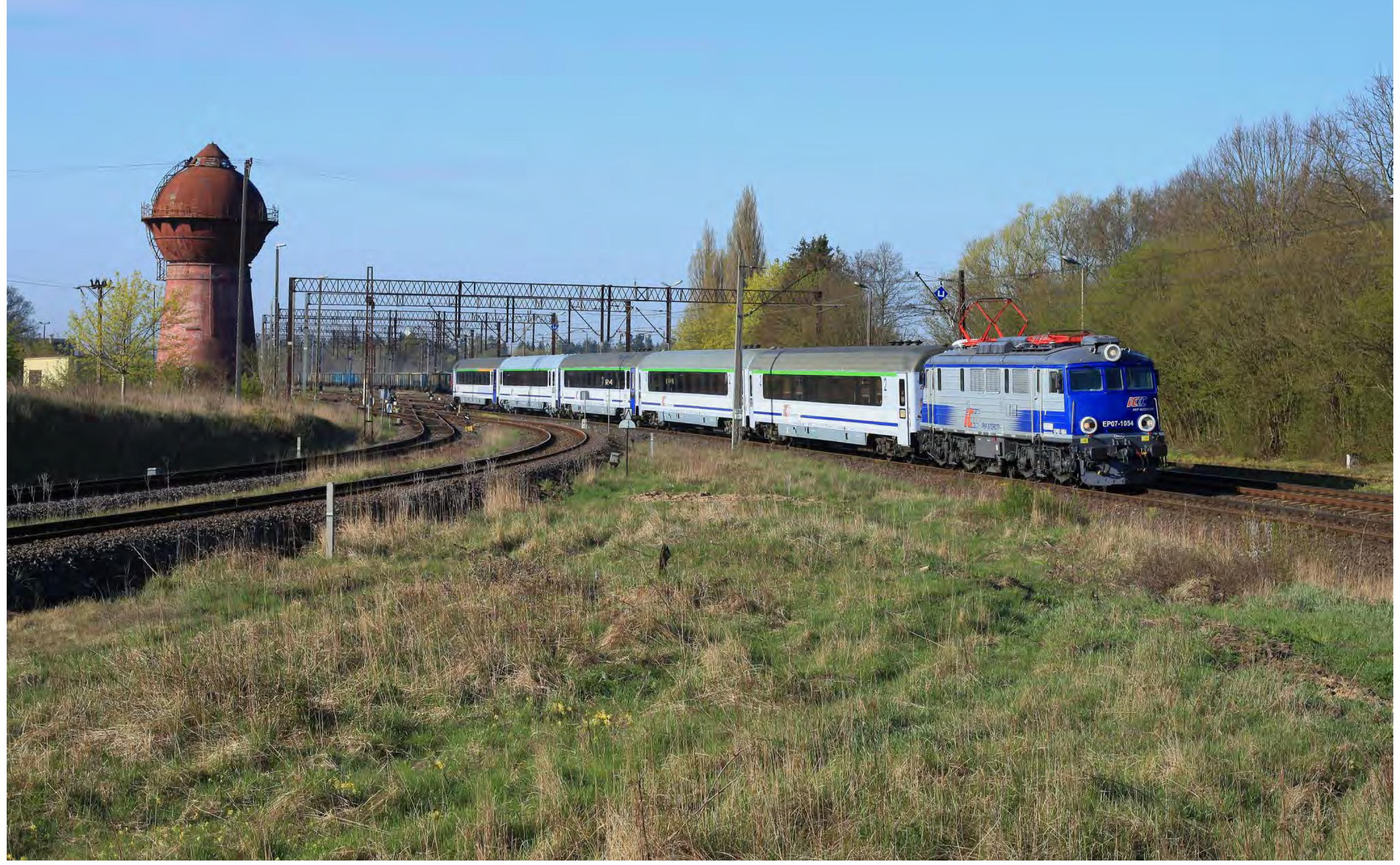
From Runowo Pomorskie is a double track non electrified mainline to Szeczinek. Even though it is double track, there are only a hand full of services a day. This is train No. R88222 hauled by a modern bi mode (diesel and electric) multiple unit, Class EN63H-003. Thomas Niederl
