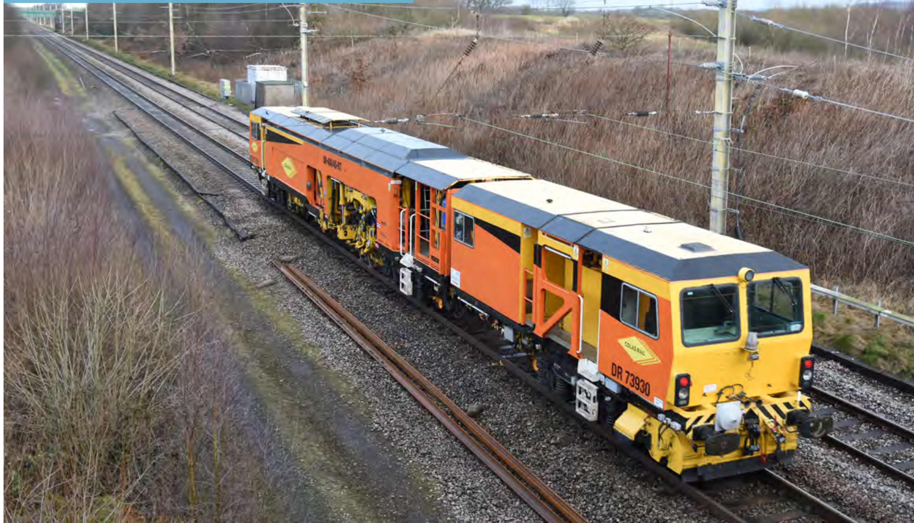
Colas Rail operated Plasser & Theurer 08-4x4/4S-RT Switch & Crossing Tamper No. DR73930 passes Bradley on February 4th. John Sloane
