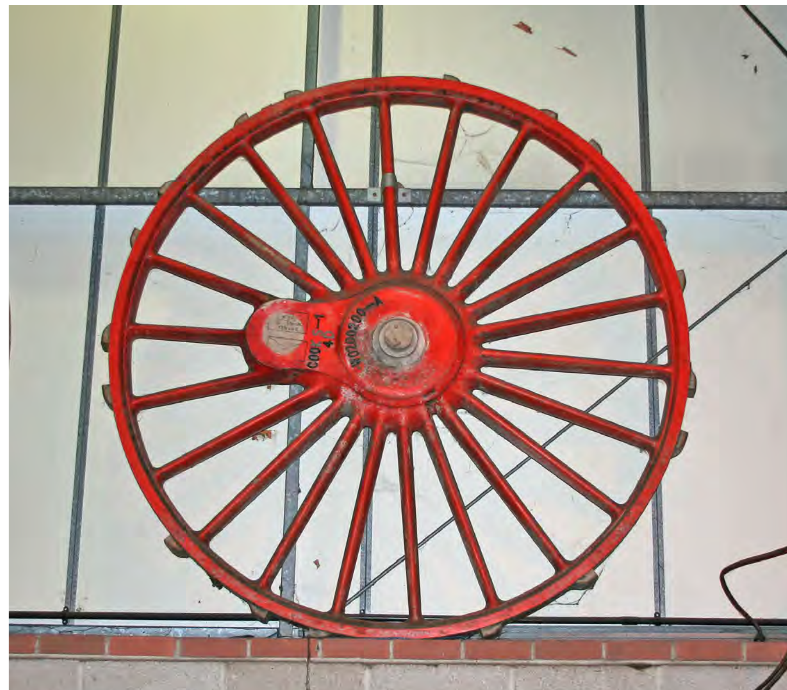
Photo: The wooden pattern for No. 3840's coupled wheels has been loaned to the Churchward County Trust by the Great Western Society, having previously been used to cast the wheels for 'Saint' 4-6-0 No. 2999 Lady of Legend. © CHURCHWARD COUNTY TRUST
