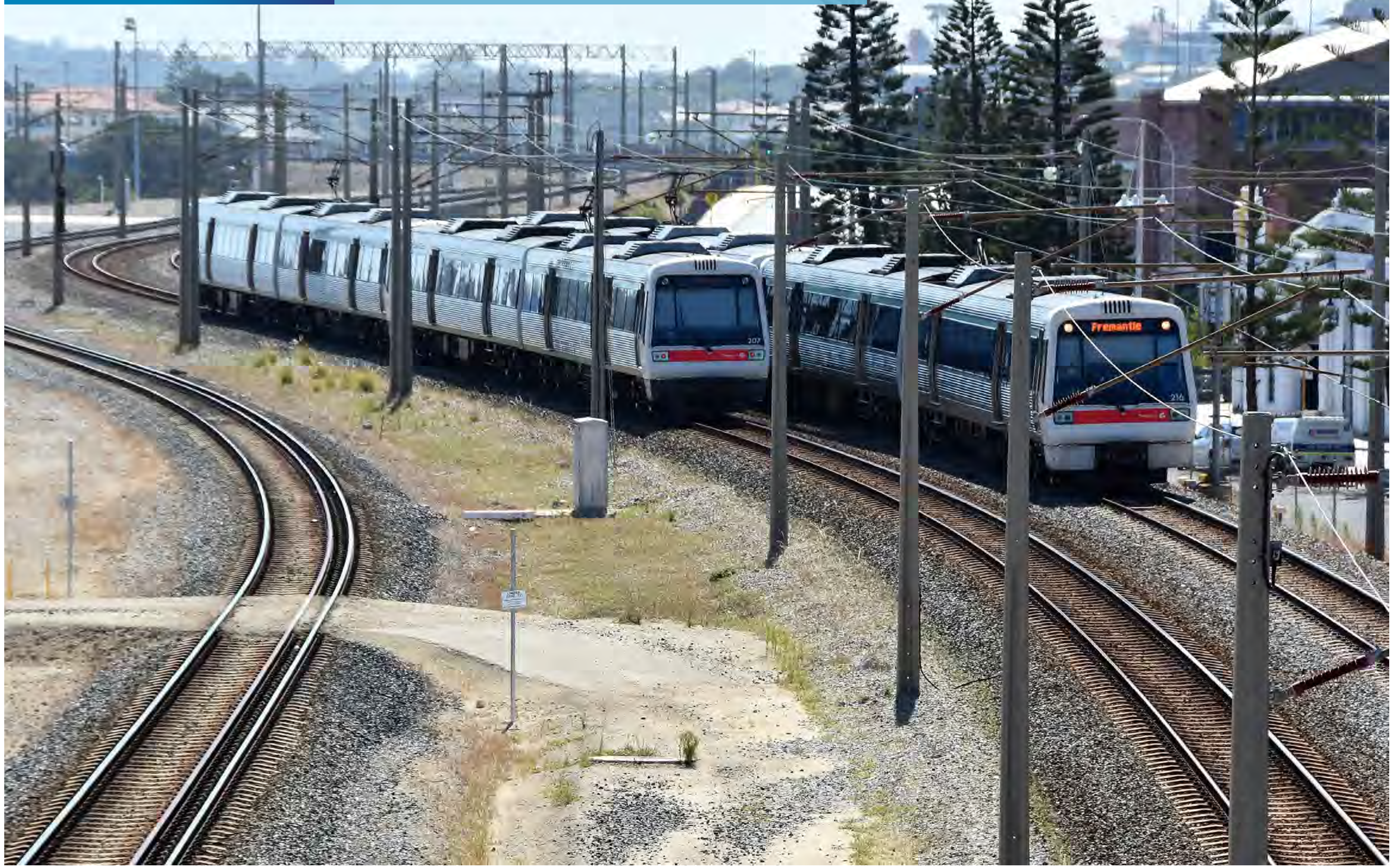
Two of Transperth's A series units pass just outside of the terminus station of Fremantle. The dual gauge track to the left is the freight only line to and from the Fremantle container port. Colin Gildersleve
