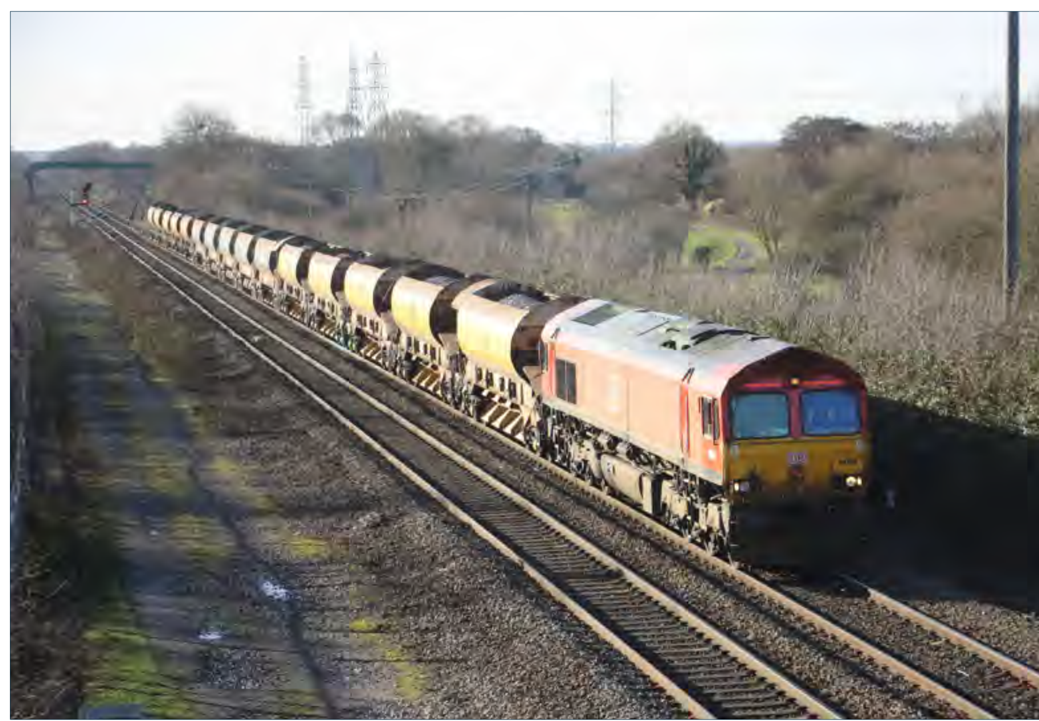
▶ Class 66 018 with 6D44 Bescot - Toton engineers train comprising of Network Rail tippers loaded with ballast, passes Stenson on January 17th. Stuart Hillis
