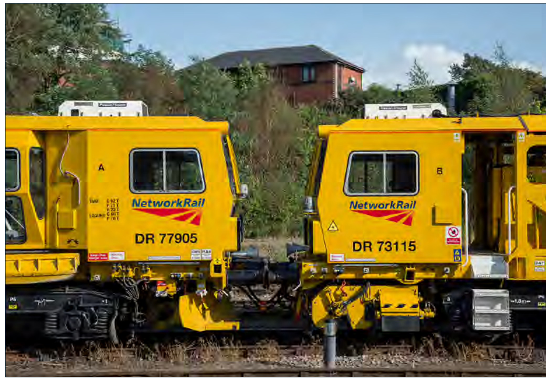
Network Rail's Type USP 5000 RT Ballast Regulator No. DR77905 and Plasser & Theurer Tamper No. DR73115 are seen stabled at Leicester on August 25th. Richard Hargreaves
