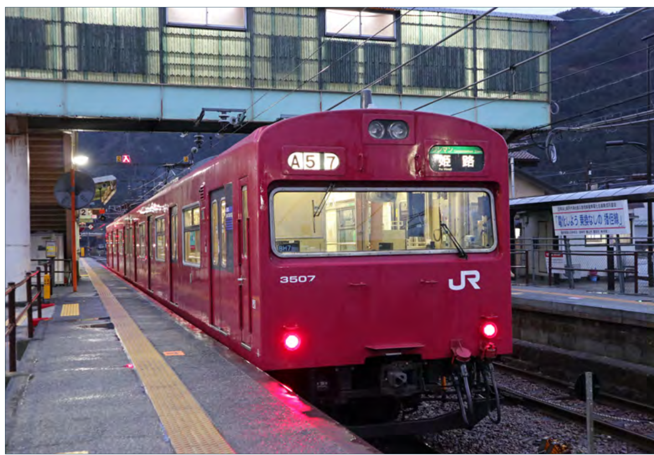
Waiting departure from Teramae on March 8th with service A57 the 18:06 to Himeji is Banton Line 2-car series 103 1500V DC 2-car EMU set BH7 formed of (DMSO) KuMoHa No. 103-3507 and (DMSOL) KuMoHa No. 102-3507 (nearest at rear). David Pollock
